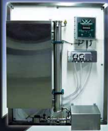
Pasteurizer Control Center Assembly
