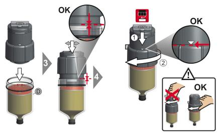
3-4 Insert control drive into grease carbridge and sits flush as shown seats onto pivot gear inside cartridge and sits flush as shown Insert control drive into grease cartridge and ensure gear drive in detail rendering above before sliding down collar and screwing onto cartridge. Rotate orange collar until indicator arrows are fully visible.
