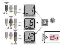
**SET UP**To select cartridge size and replacement interval, hold the "SET" button for 5 seconds until three size bars begin to flash in display. Press "SET" button until horizontal line corresponds with appropriate cartridge size. Release "SET" button until monthly interval digit flashes, then click the "SET" button until the appropriate monthly service interval matches the cartridge size indicated by the chart at left. Once monthly interval and cartridge size
