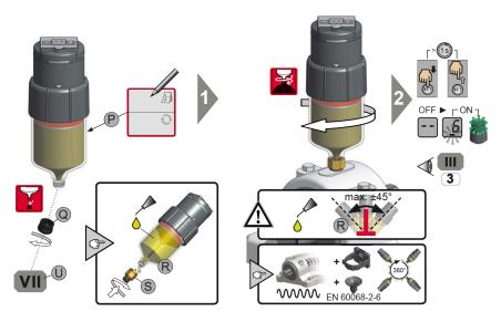
After writing installation date on the cartridge label, screw **ALL** into grease fitting at no more than a 45 degree angle. Click "SET" button to turn on unit and watch for green flicker light at the top of the unit. When empty or in the event of a low battery, unit will flicker red. Reinstall clear protective cover.
