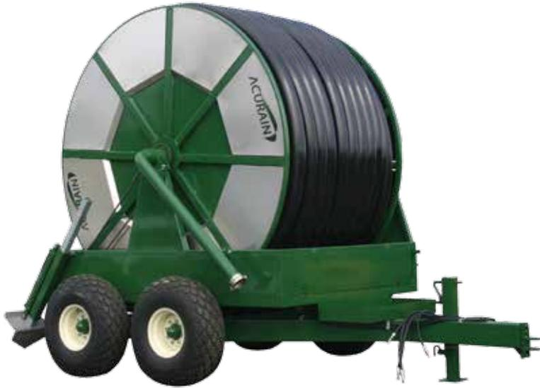
Dragging hard hose has many advantages over the traditional method of soft hose. Including: longer life, quicker hose retrieval, less hose twisting and easier pulling. Couple this with sturdy construction of the chassis, and you can stretch your investment dollars further. Our Acurain 4500M has 1320' of 5.512" OD X 0.591" wall HDPE hose that can cover over 65 acres in a single set.
