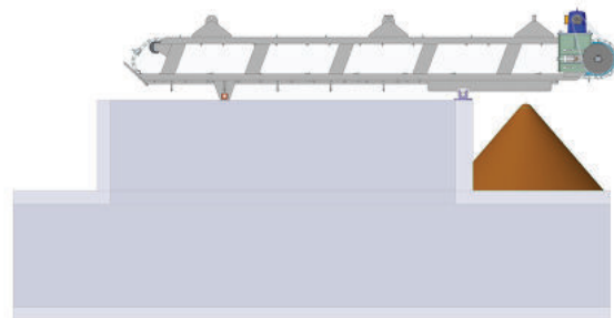
Lifted on rotating pivot for service
