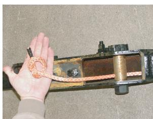
(5) Pick up slack and tie off with overhand knot and cut off end
