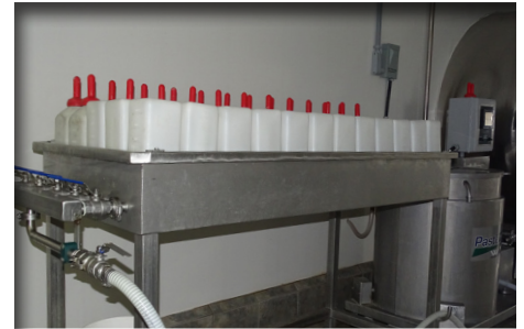
Easy loading grid features cone spray nozzles for clean spray and excellent bottle coverage.
