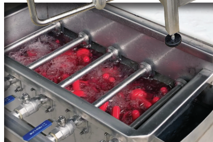
Washer jet rails and water flow clean and sanitize nipples during the bottle wash cycle.
