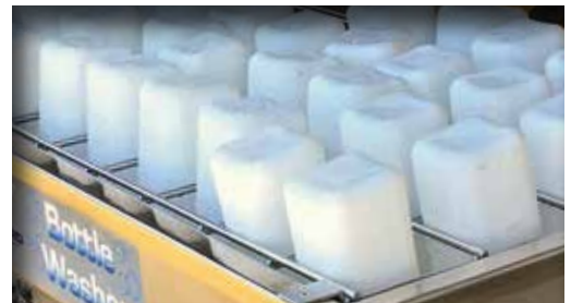
Easy loading grid features cone spray nozzles for clean spray and excellent bottle coverage.
