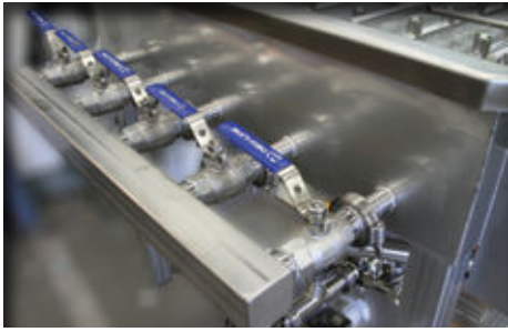
Individual valve zone control for washing at less than full capacity.
